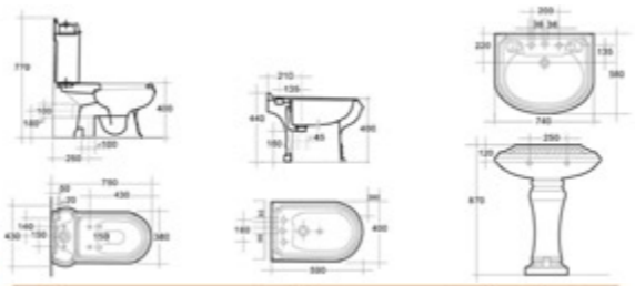
CZU-7011 CZU-7012 CZU-7013 Washdown Close-coupled Closet Bidet Washbasin with pedestal Size: 750x430x770 mm Size: 590x400x440 mm Size: 740x580x870 mm
