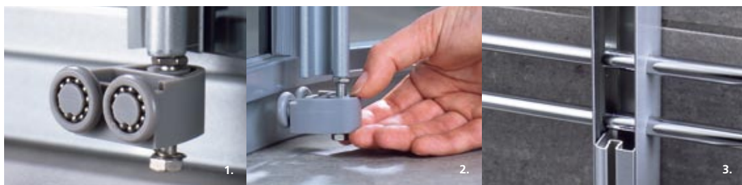
1, 2. Each door has sprung bogie carriages with ball bearings that allow the door to slide smoothly and quietly. Spring mounting makes it easy to release the bottom of the door for cleaning. 3. Exposed pipes are not a problem. They can easily be run through the aluminium profile.
