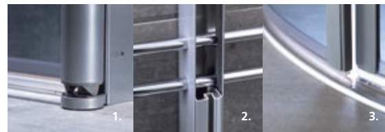
1. Neat hinges lower the door as it closes, compressing the rubber seal against the floor. 2. Exposed pipes are not a problem. They can easily be run through the aluminium profile. 3. If the floor slopes the wrong way, a radius strip can be fitted to the floor to prevent water escaping. Strips: Entré round 70x90, 80x80 and 90x90. Entré straight
